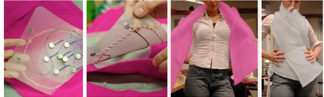
Figure 1: the Affective TouchCasting prototype showing flexible haptic I/O modules (left) in a discrete fashionable scarf (right).
